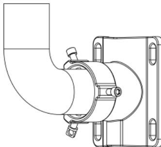
2. Connect one side of the sensor cable to the WTS Sensor and tighten the cable, pass the cable through the bent pipe and bracket, then connect the pipe to the bottom of the sensor and fix both parts with 3 hex socket cap mounting screws.
