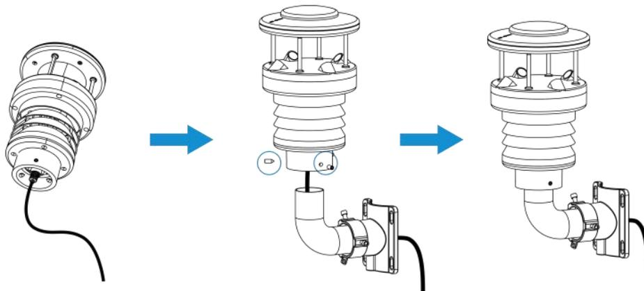
3. Straighten the hose clamps and slide them through the rings in the bracket, wrap the hose clamps around the pole. After that use a screwdriver to tighten the locking mechanism by turning it clockwise. When installing, ensure the arrow on the sensor facing north according to a compass.
