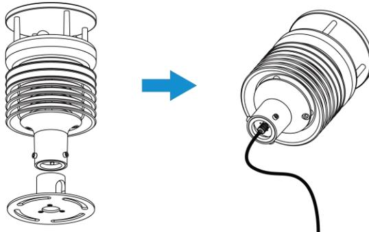
2. Connect the sensor to the pole top flange with nuts and bolts, then connect the other side of the sensor cable to the right interface of the WTS Hub. When installing, ensure the arrow on the sensor is facing north according to a compass. Users can install the sensor with other installation methods by selecting other accessories.
