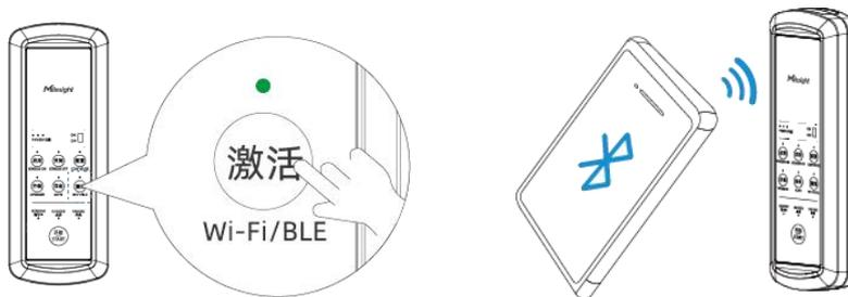
4. Basic information and settings of devices will be shown on ToolBox App if it's connected successfully. Go to **Settings** page to click **Upload files** button to select and upload firmware from smartphone. **Every SCT01 device can only save one firmware file.**
